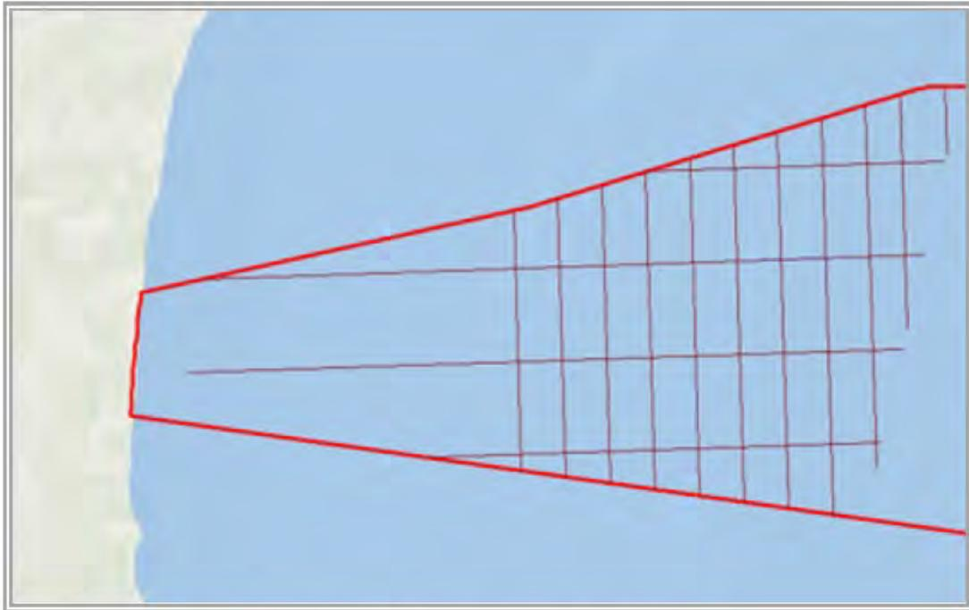
**Figure 3: Survey lines acquired (inshore section)**
