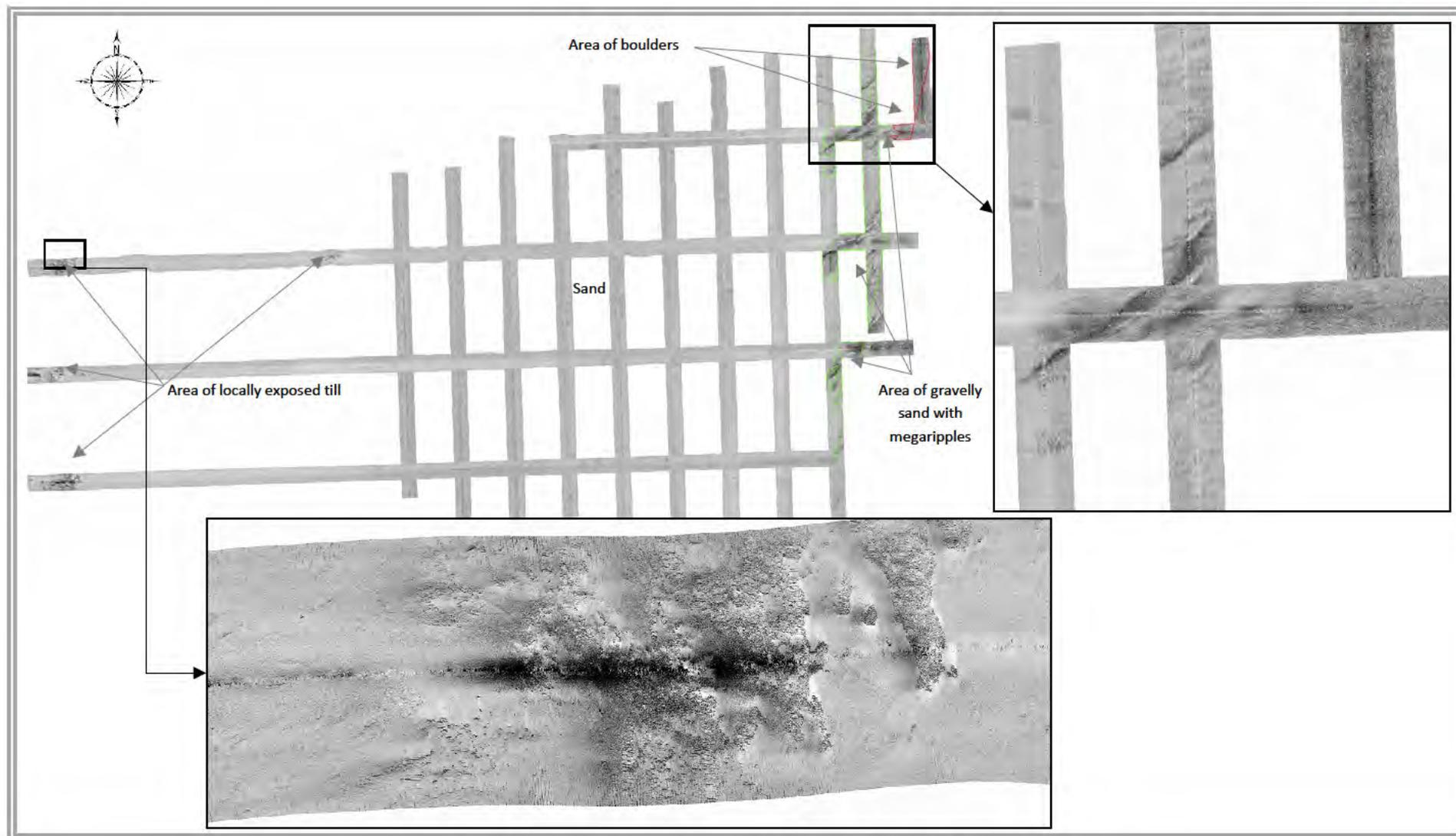
**Figure 9: Seabed Features – Areas of Till, Gravelly Sands and Boulders**
